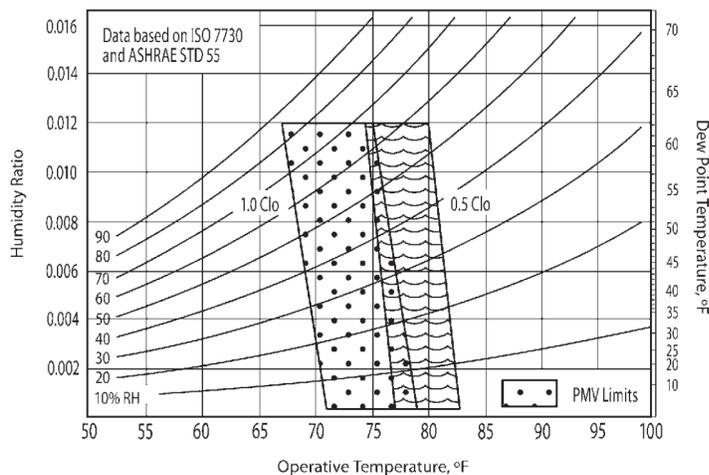
Figure 1. Static Model Psychrometric Chart displaying two zones of comfort that account for clothing worn in both warm and cold outdoor air temperatures from “Mechanical and Electrical Equipment for Buildings” (Grondzik et. al. 2019)
